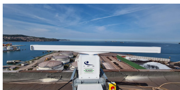
A radar for detecting pollution at sea, installed on the roof of a silo in the port of Koper.
